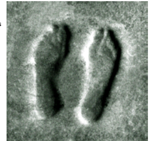
An example of "memory" These footprint impressions in a Pudgee cushion remain several seconds after the person who made them has left.
