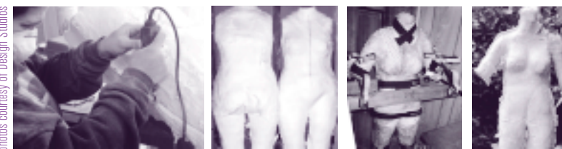
Left to Right: prepping the plaster cast; back and front halves of cast; preparation for pour; foam mannequin immediately after mold is removed.
